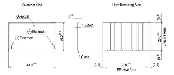
Note: Glass Substrate Thickness : 1.1mm Module Thickness : 1.3mm max
